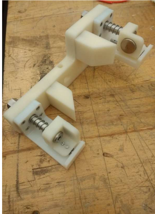
Figure 99: Assembled magnet handoff mechanism
